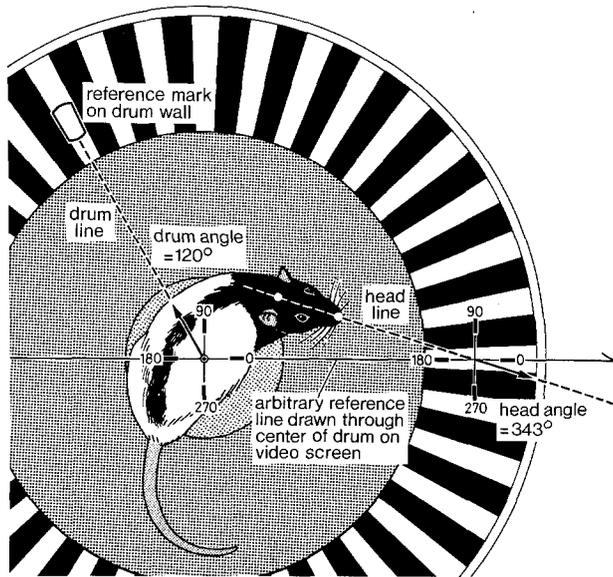
Fig. 1. Diagram indicating how drum and head angular position in space were measured on still frames of video records of responses to optokinetic stimulation. See text for details
